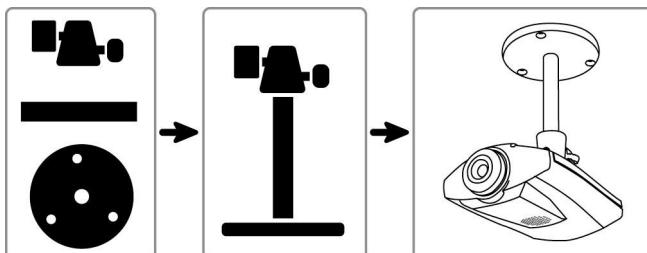
Step1: Fasten the base of the bracket (the round one) to where the camera is installed.
