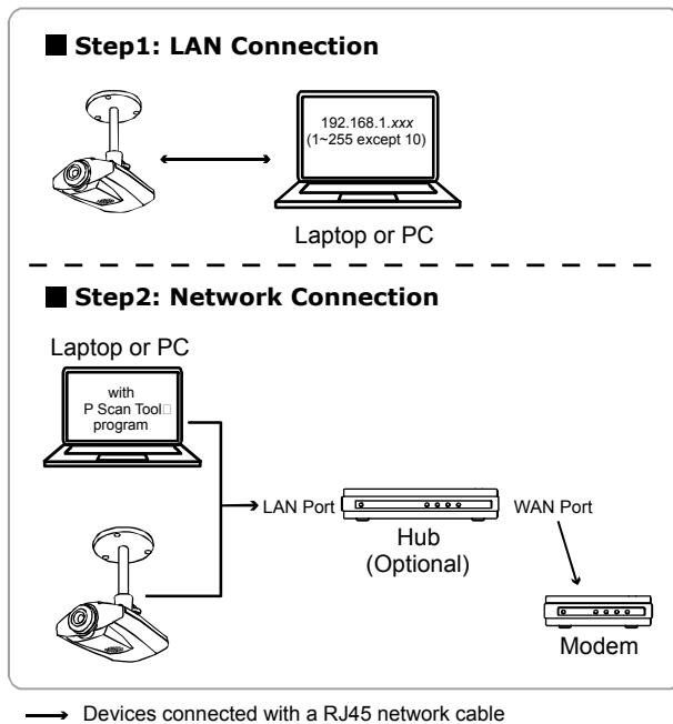
Step1: Disconnect your laptop / PC from the hub or modem, and connect it to this camera with a network cable.
